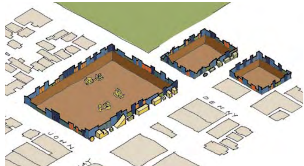
Figure 8.1 Construction Mitigation - Interim Diagram
